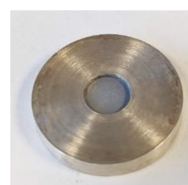
Pressed ^{135}\text{Ba}[\text{BaCO}_3]/\text{Al} target (1/2, w/w) 200 mg
