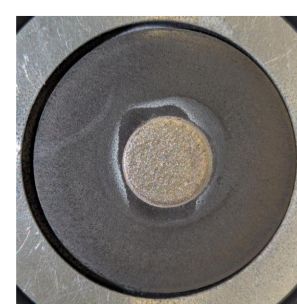
Target after irradiation ^{103}\text{Pd} yield 2.0 \pm 0.6 MBq/ \mu\text{Ah}
