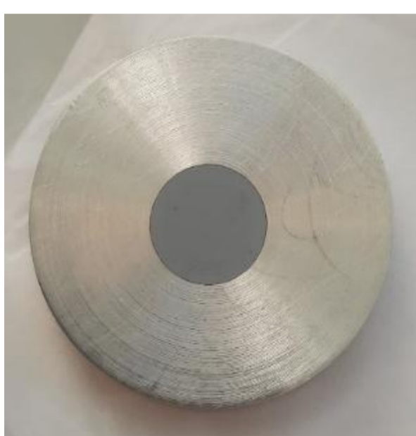
Electroplated ^{\text{nat}}\text{Cr} target 50-58 mg
