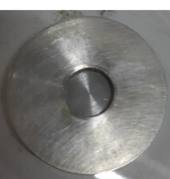
Pressed ^{\text{nat}}\text{Ho}_2\text{O}_3/\text{Al} target (1/1, w/w) 180 mg
