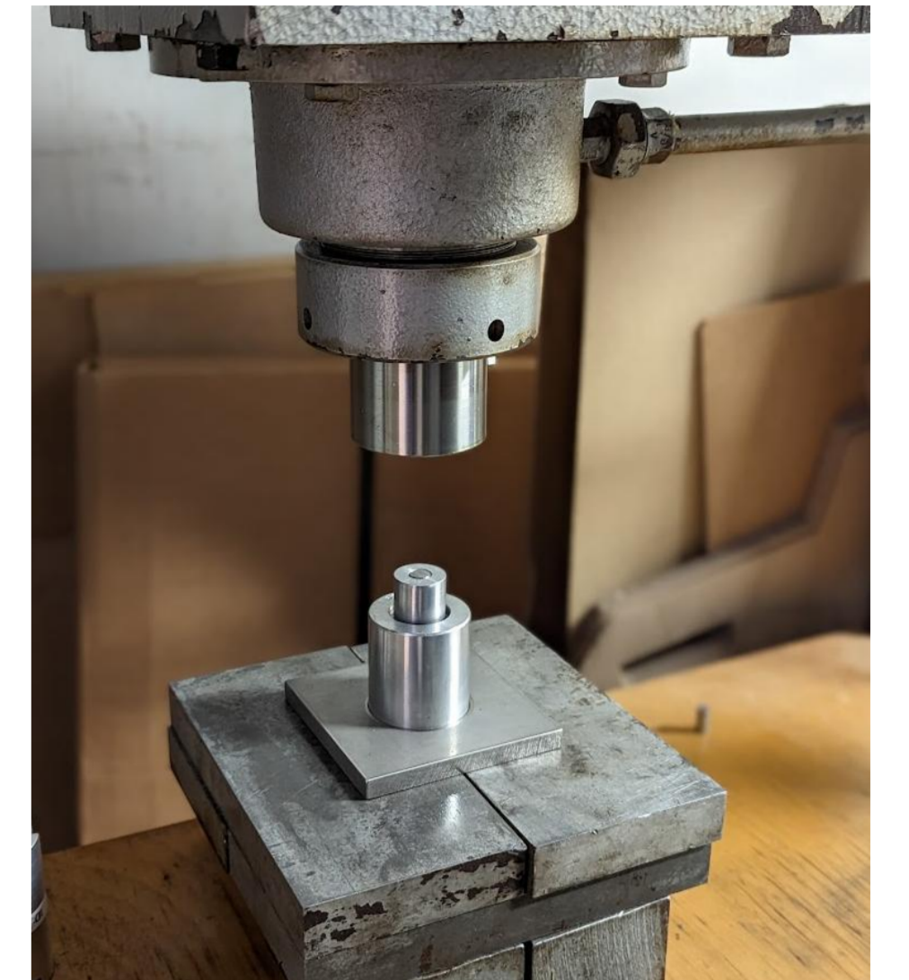
Hydraulic press with stainless steel piston and anvil
