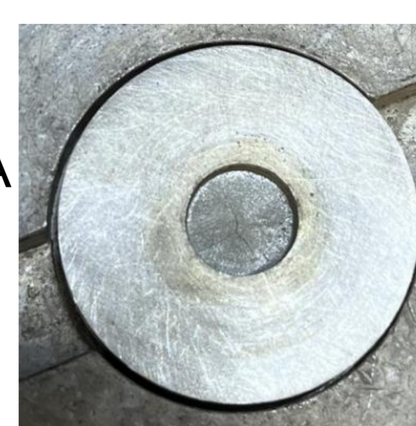
Target after irradiation ^{165}\text{Er} yield 12.5 \pm 1.6 MBq/ \mu\text{Ah}
