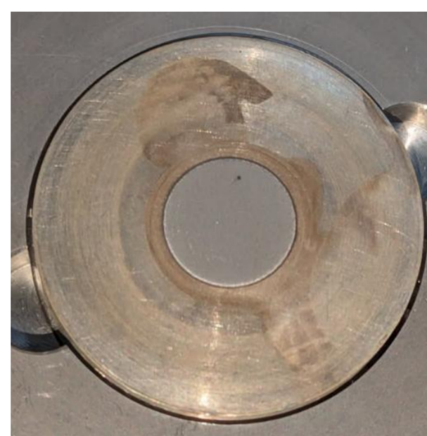
Target after irradiation ^{52}\text{Mn} yield 2.3 \pm 0.2 MBq/ \mu\text{Ah}
