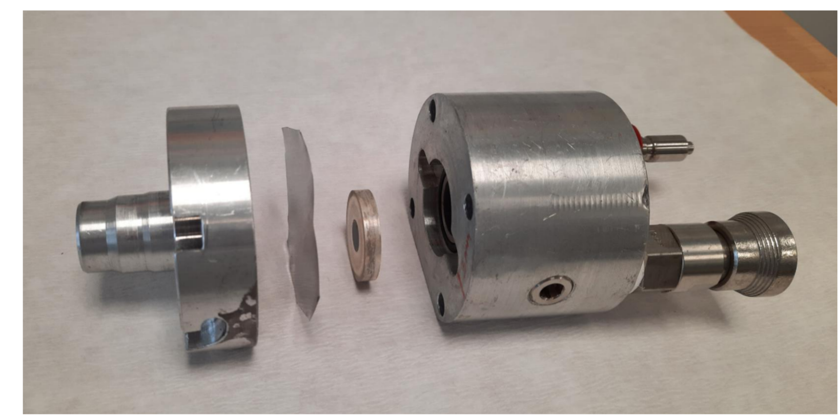
Target body showing degrader foil and target on backing
