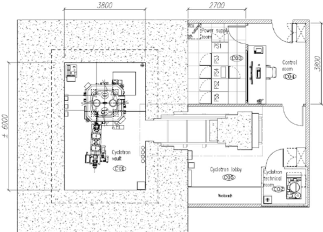
Figure 23: Cyclone® KIUBE with short beam line (vault)
