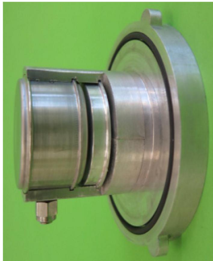
Figure 6. The tandem Rb/Ga targets mounted on a bayonet-mount plug.
