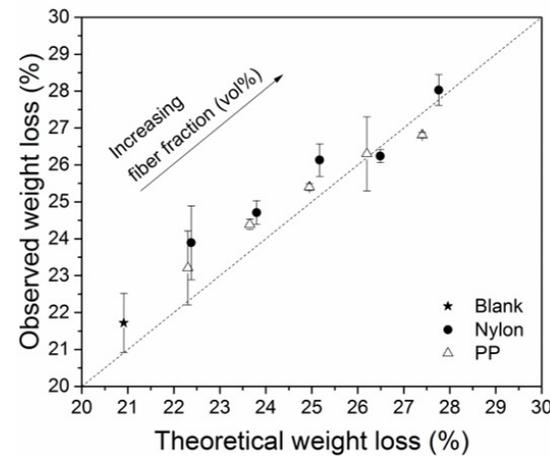
Fibers allow to obtain similar permeability but with lower vol% of filler (lower total porosity) with respect to PMMA microspheres
