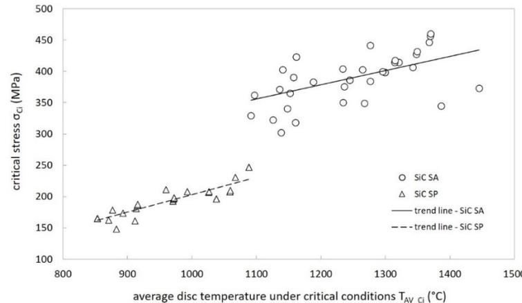
Obtainable data: critical stress under irradiation, probability of survival under irradiation without undergoing failure
