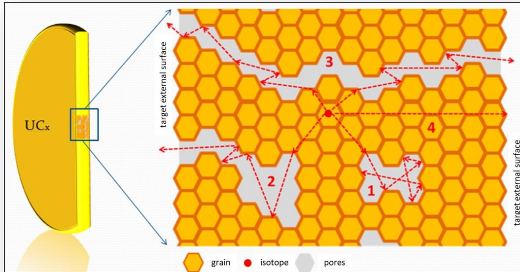
**Open porosity and nanostructure to obtain fast release of isotopes**
