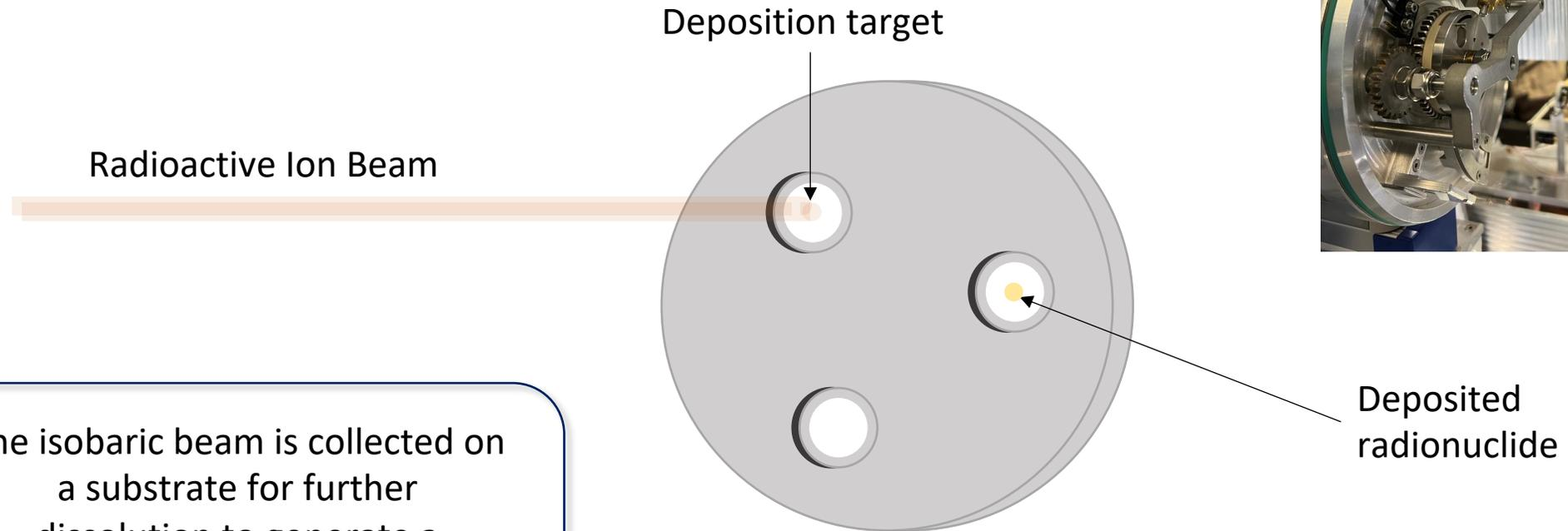
The isobaric beam is collected on a substrate for further dissolution to generate a solution for radiolabelling of pharmaceuticals
