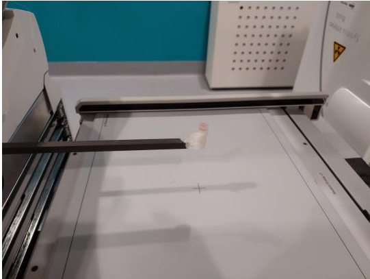
Figure 1: setup for peaking the energy spectrum for ^{225}\text{Ac}
